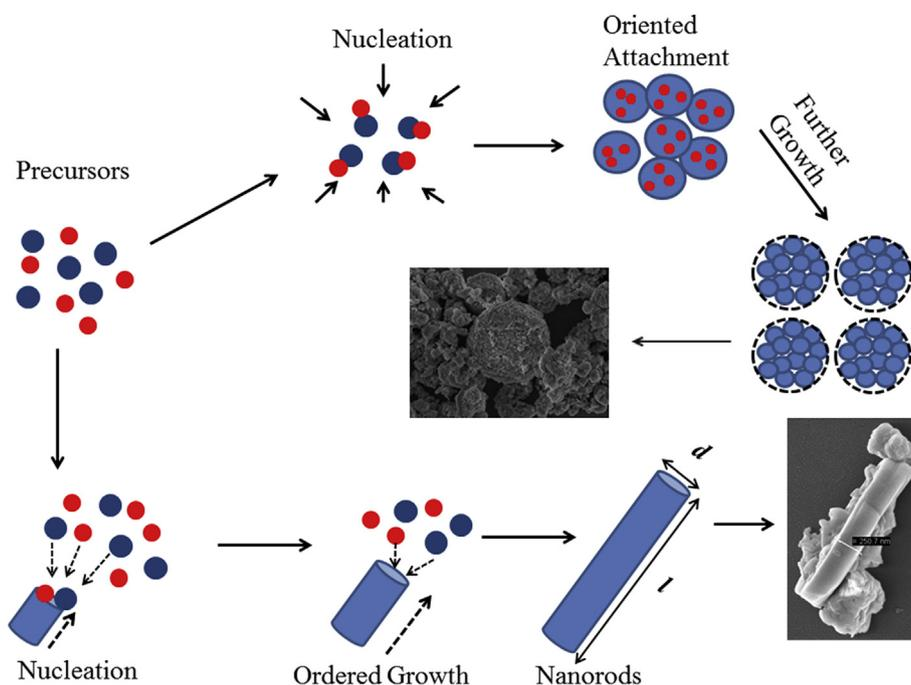
Fig. 3. Schematic illustration for the possible formation of microspherical mechanisms and nanorods of ZnMoO<sub>4</sub>.
