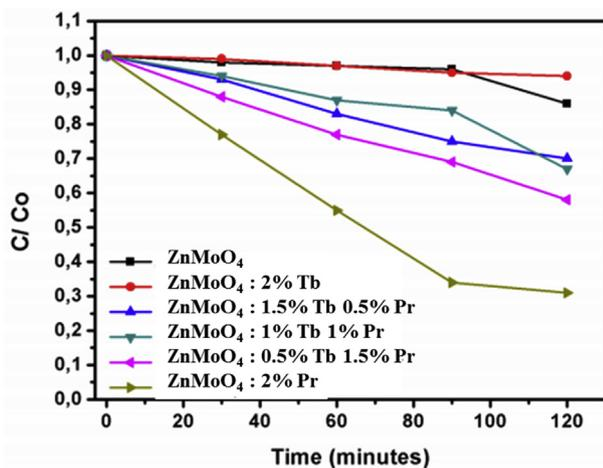
Fig. 10. Variation in the concentration of the methylene blue dye against the synthesized ZnMoO<sub>4</sub>:Tb<sup>3+</sup>, Pr<sup>3+</sup> powders submitted to UV radiation. (For interpretation of the references to color in this figure legend, the reader is referred to the Web version of this article.)
