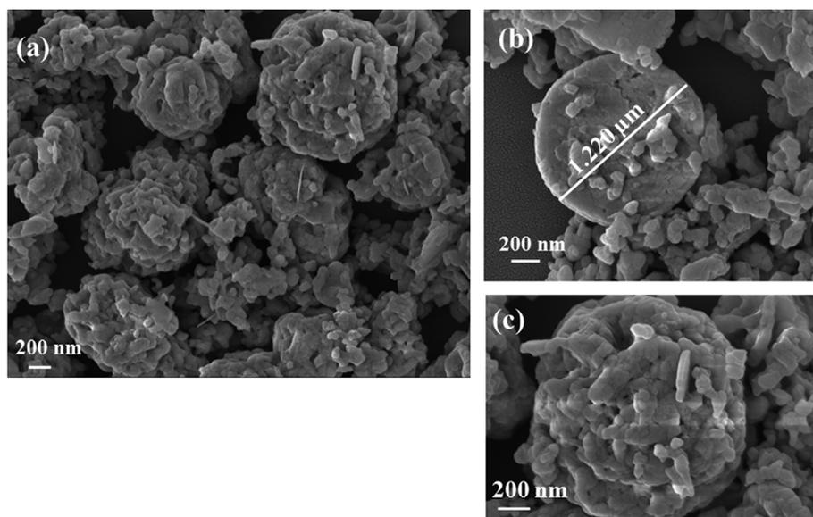
**Fig. 2.** FEG-SEM micrographs of  $\text{ZnMoO}_4$  and  $\text{ZnMoO}_4:\text{Tb}^{3+}$ ,  $\text{Pr}^{3+}$  particles prepared by the sonochemical method,  $\text{ZnMoO}_4$  (a–c),  $\text{ZnMoO}_4:2\% \text{Tb}^{3+}$  (d–f),  $\text{ZnMoO}_4:2\% \text{Pr}^{3+}$  (g–i).
