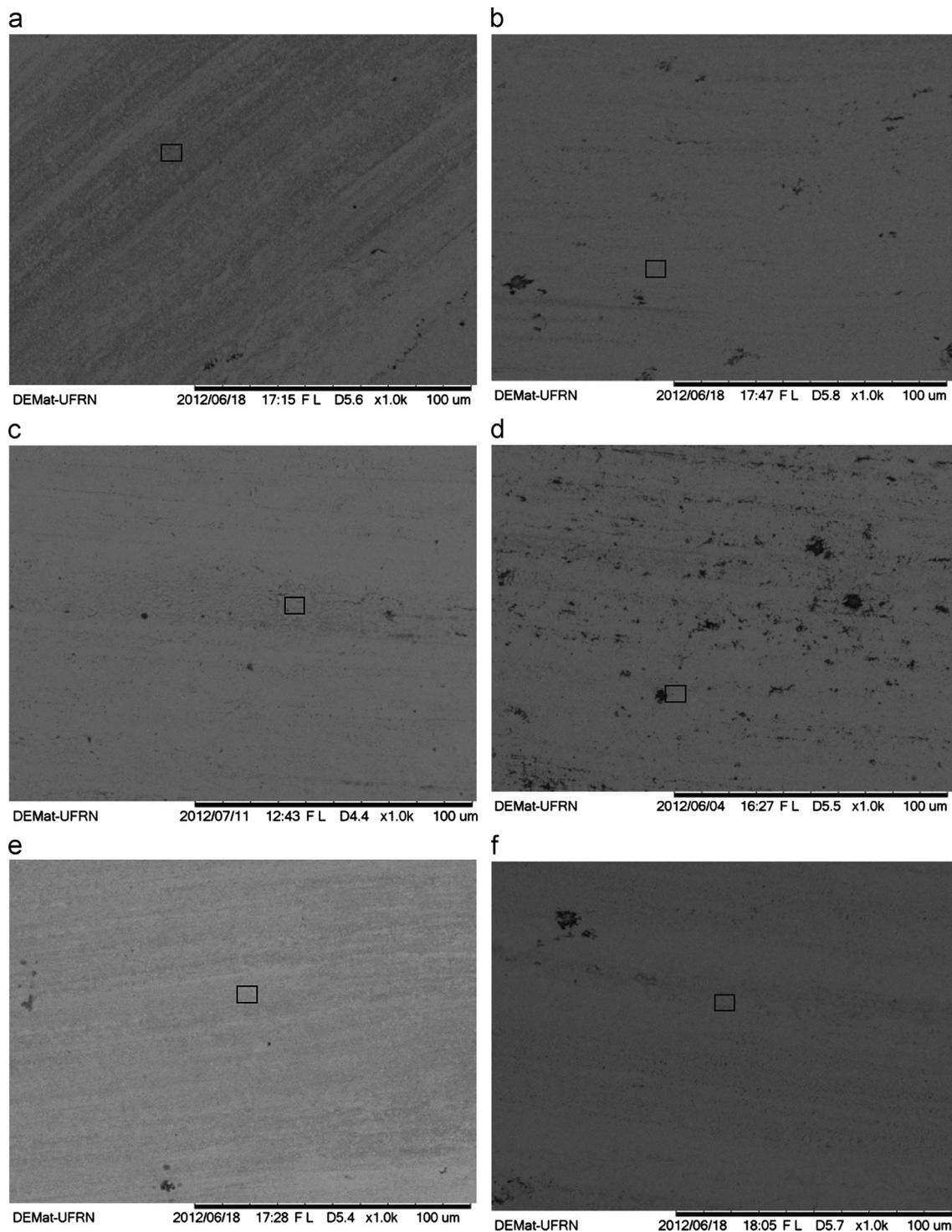
**Fig. 6.** SEM micrographs of the worn surfaces lubricated with: (a) sunflower oil (WSD =  $187.5 \pm 0.7 \mu\text{m}$ ) (b) soybean oil (WSD =  $203.5 \pm 0.4 \mu\text{m}$ ) (c) sunflower oil+CuO (WSD =  $198.5 \pm 4.9 \mu\text{m}$ ) (d) soybean oil+CuO (WSD =  $230.2 \pm 1.1 \mu\text{m}$ ) (e) sunflower oil+ZnO (WSD =  $202 \pm 1.4 \mu\text{m}$ ) and (f) soybean oil+ZnO (WSD =  $240.5 \pm 2.1 \mu\text{m}$ ).
