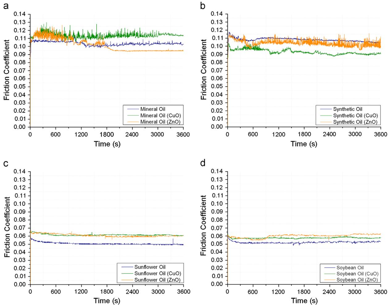
**Fig. 4.** Friction coefficients as functions of time lubricated with different oil base without and with nanoparticles additive: (a) mineral oil, (b) synthetic oil, (c) sunflower oil and (d) soybean oil.
